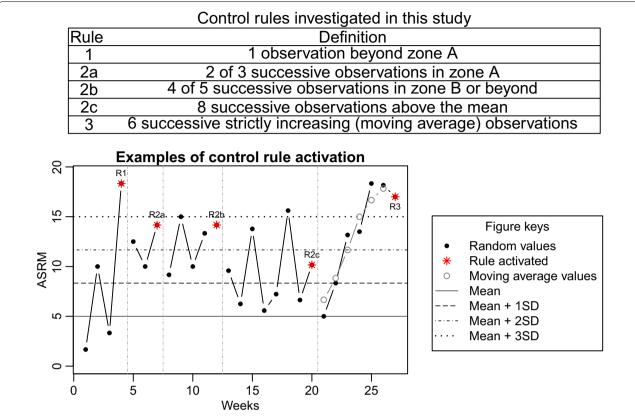
**Fig. 3** Control rules investigated in this study and examples of control rule activation. ASRM scores were randomly generated with mean = 5 and SD = 3.3. Independent sections where each of the five control rules investigated in this study was activated are shown. A control rule was said to be activated on the observation by which all its conditions were satisfied
